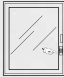
Casement windows: Fit lock in the middle.
